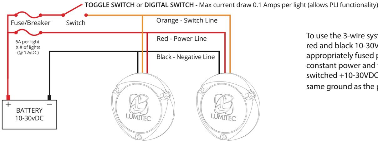
To use the 3-wire system, simply connect the red and black 10-30VDC lines to an appropriately fused power buss with constant power and the Orange wire to a switched +10-30VDC buss referenced to the same ground as the power lines.
