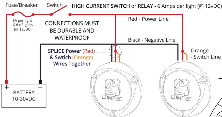
NOTE: The SBX2 can also be wired in a standard two wire installation as well by simply connecting the red and orange wires together and powering via an appropriately rated switched power buss.
